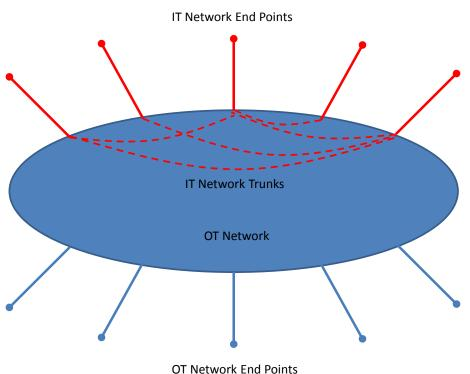
Figure 1: Logical Separation between OT and IT Networks
