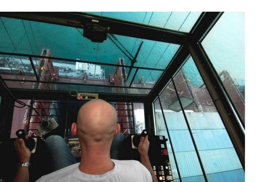
For all the advantages over diesel, electrical automation puts much more demand on a port's power supply. Traditional quay cranes often have peak demands of around 2000kVA. While a typical automated stacking crane (ASC) may only peak at 50% to 60% of that, an automated terminal could easily be looking at two or three dozen of them – so drawing several tens of thousands of kVA when operating a full stretch.
